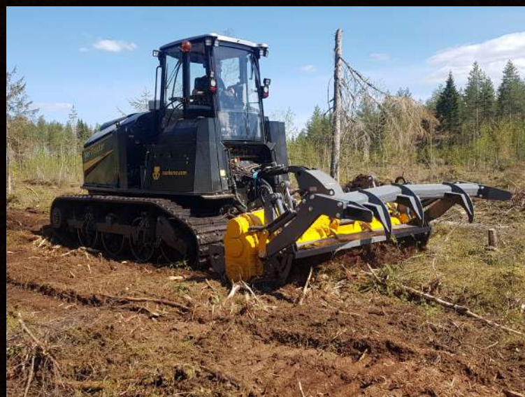
MT-700 with rubber tracks and MJHS 3.1 meter crusher reclaiming soil after harvesting before replanting
