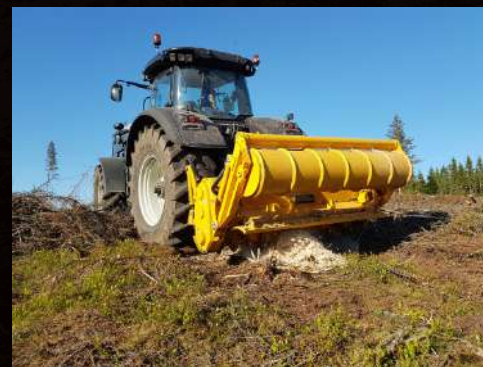
MJS crushing stumps after logging
